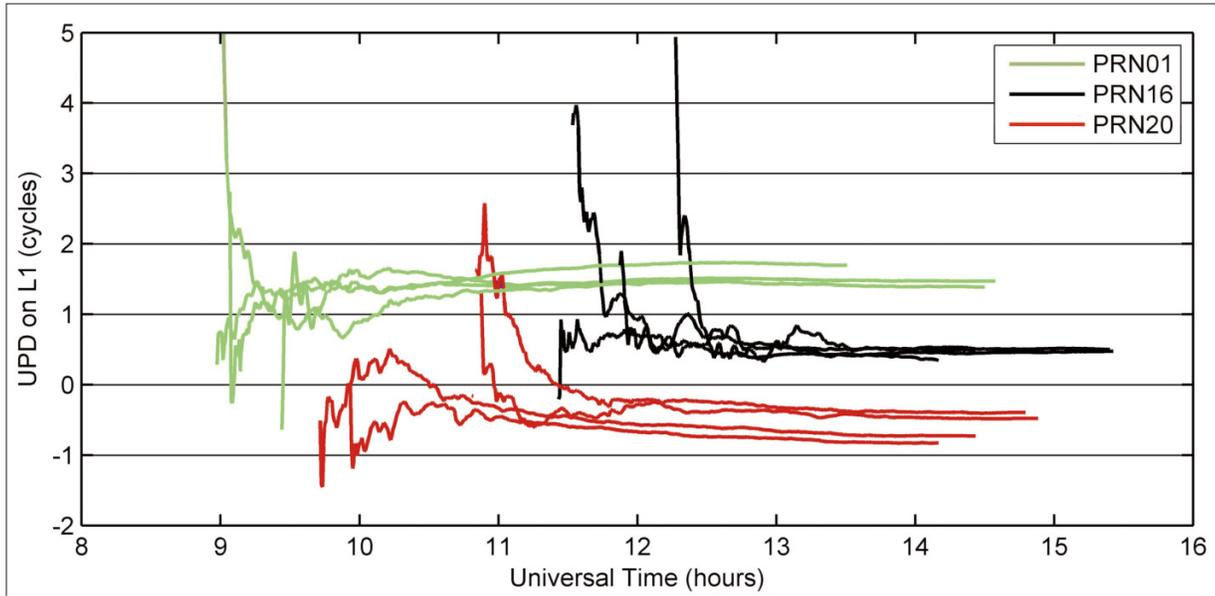
Figure 5: UPD on L1 for selected satellites calculated with four stations through Canada, October 17, 2007 / Biais de phase sur l'onde porteuse L1 calculés à partir de quatre stations à travers le Canada, 17 octobre 2007.
